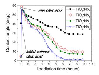
Fig. 3.2 Modification of the contact angle after depositing the oleic acid layer, and its variation as a function of the irradiation time
