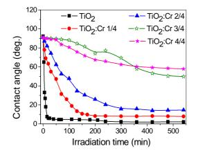
**Fig. 3.7** Contact angle as a function of the irradiation time for the  $TiO_2$  films having different Cr percentages
