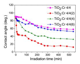
Fig. 3. 8 Contact angle as a function of the irradiation time for the  $TiO_2$  films with the highest Cr concentration ( $TiO_2$ :Cr 4/4), having different Pt islands deposited on their surfaces
