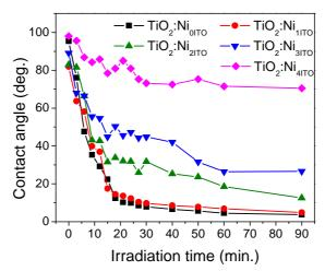
Fig. 3.6 Contact angle as a function of the irradiation time for the sample deposited on ITO/glass substrate
