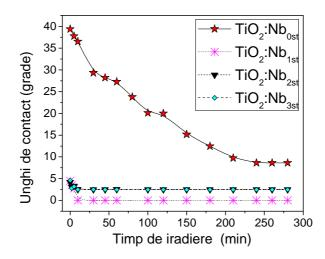
Fig. 3.1 Contact angle vs. UV irradiation time plots for the pristine  $TiO_2$  and  $TiO_2/Nb$  samples
